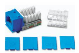
Designed for superior performance, this keystone jack is available in 9 colors to match housing or allow color-coded port designation in compliance with TIA-606 requirements. Includes 110-type IDC termination with strain relief caps, and comes standard with 50 inch gold plating on the jack contacts.
