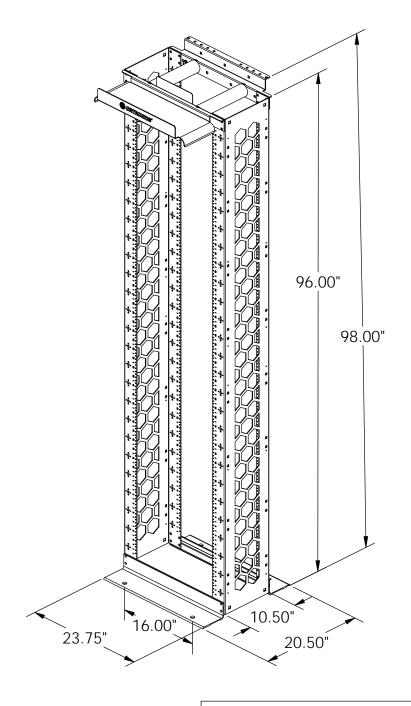
TESTED TO UL2416 WITH A WEIGHT LOAD OF 2000LBS.
