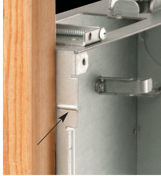
Positioning tabs are set for 1/2" or 5/8" drywall.
