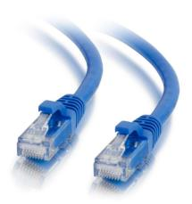
This Snagless Unshielded Catóa patch cable is ideal for use with 10GBase-T ports and equipment, such as network adapters, hubs, switches, routers, DSL/cable modems and patch panels, and enables 10 Gigabit data transmission over a 4 pair copper cable allowing connections up to 100 meters. Current Cat6 cabling systems may only support 10 Gigabit Ethernet over limited distances. Each patch cable is fully tested to meet ANSI/TIA 568 C.2 Cat6a channel requirements.
