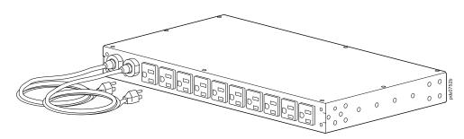
**Input power cords:** Two (2) cords connect the Rack ATS to two separate power sources (A and B). The Rack ATS draws power from the preferred source and automatically switches to the secondary source when necessary. The two (2) 2.44-m (8-ft) power cords have NEMA 5-15P plugs.
