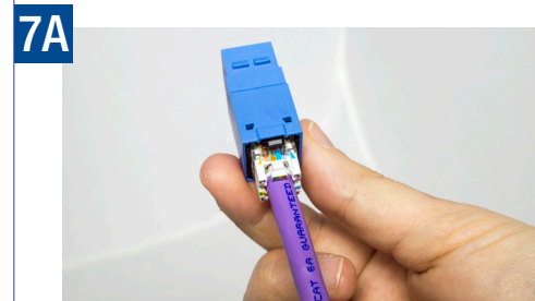
After cable is fully prepped, align your pairs in a 2 up, 2 down formation T568A: Green and brown pair up T568B: Orange and brown pair up
