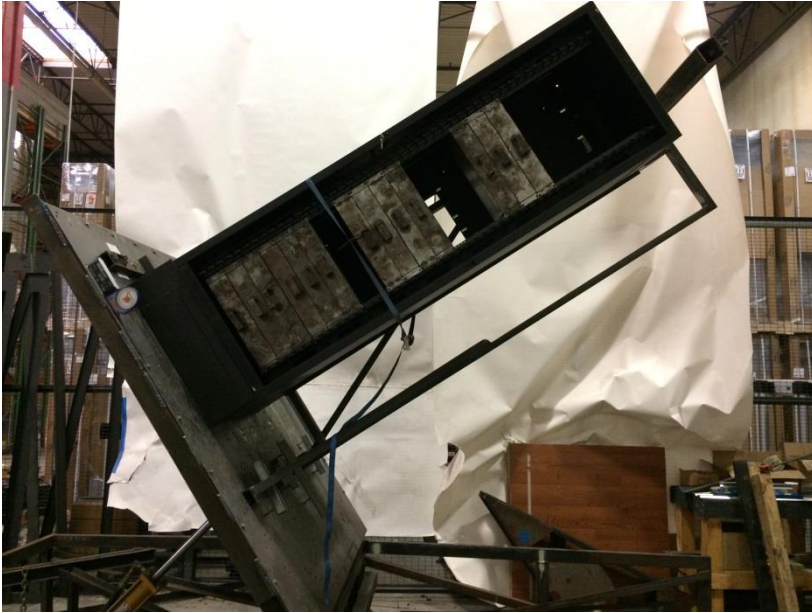
Photo 3 SR-46-32 at maximum inclination in side-to- side direction
