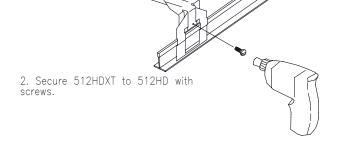
Note: 512HDXT provides 3-5/8" spacing from face of tile to bottom of bar to accommodate 2-1/8" box with 1-1/2" extension ring.
