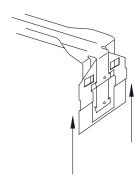
1. Slide 512HD onto the 512HDXT making sure the extension legs are under then bent arms.
