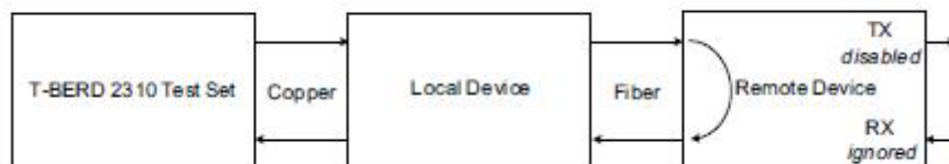
Figure 22: Initiate a Loopback from a Test Set
