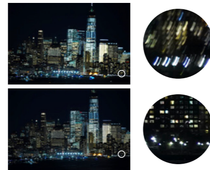
Compensation for roll shake on the Z-axis during long exposures. Most in-lens systems for interchangeable-lens cameras cannot compensate for roll shake.
