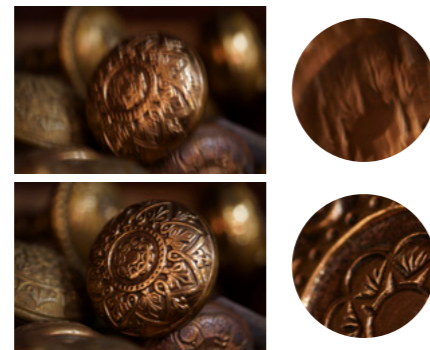
Compensation for X and Y-axis shift shake at high magnification (during macro photography, etc.).
