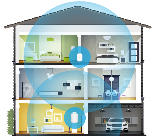
UDM on Floor 1, UniFi AP Beacon HD on Floor 3
