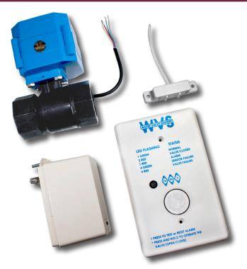
The GRI Water Valve Shutoff System was designed as a flood prevention device. This system utilizes an electronic controller to provide automatic control of an electronic water valve that is installed in the main water supply line. The controller continually monitors water sensors that are placed in areas where flooding from water line breaks are most likely to occur; washing machine, hot water heater, sinks, dishwasher.
