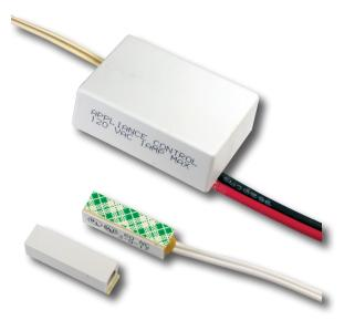
The GRI Current Controller is an encapsulated circuit with connecting wires to AC power, a light fixture and door monitor switch. A microprocessor circuit is safely isolated from the 120 volts AC. This control signal through the door switch will control the AC power to the light fixture. The GRI Current Controller is designed to fit into an electrical junction box along with the connecting wires.
