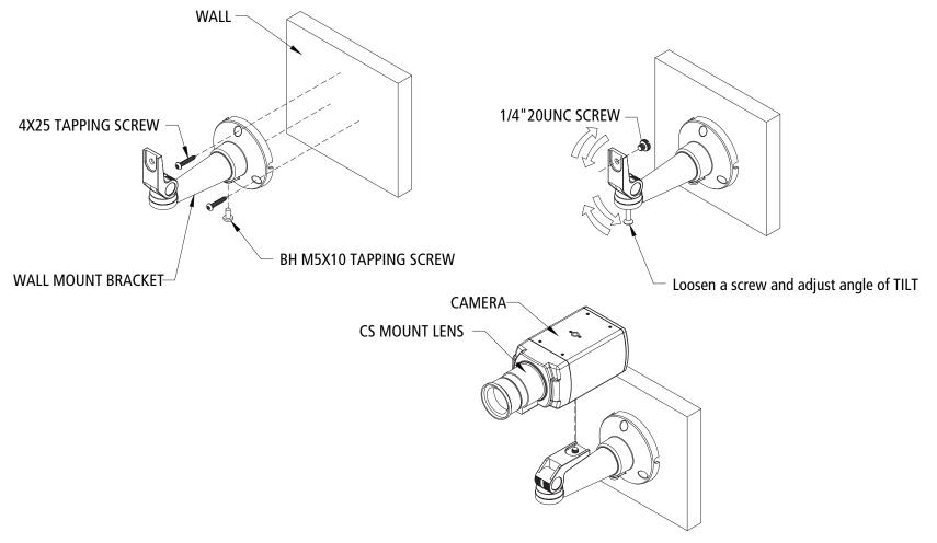
WARNING: You might need to reinforce the wall or ceiling. If the wall or ceiling is not strong enough to support the camera, the camera might fall damaging the camera or causing injuries
