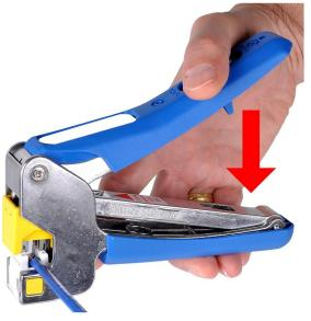
Remove the jack from the tool's receptacle.
