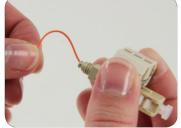
Insert the fiber into the connector with mark facing up. Create a slight bend in the fiber to maintain connection.
