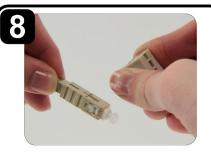
Release the wedge clip by squeezing both sides. Remove the wedge clip.
