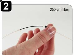
Insert the clear tubing, 250-µm tubing, and 900-µm boot onto the fiber.
