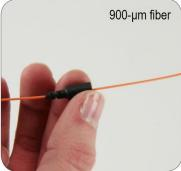
Place the 900-µm boot on the cable.
