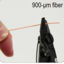
Strip 35 mm of 900- and 250-µm coating off.
