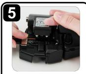
Set the fiber on the cleaver at the 10.5-mm cleave length. Cleave the fiber.
