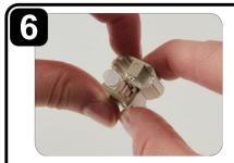
Squeeze top and bottom of the wedge to ensure that it is engaged.
