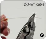
Strip off 35 mm of 900-µm and 250-µm coating.
