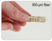
Slide the boot onto the connector body. Termination is complete.
