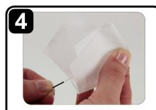
Clean the fiber with a lint-free wipe and fiber preparation fluid.
