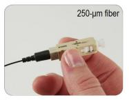
Slide the boot onto the connector body. Bring the clear protective tubing over the end of the 250 µm protective tubing. Termination is complete.
