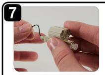
Insert fiber into connector. Bring 250  $\mu$ m protective tubing forward. Create a slight bend in the fiber to maintain connection.
