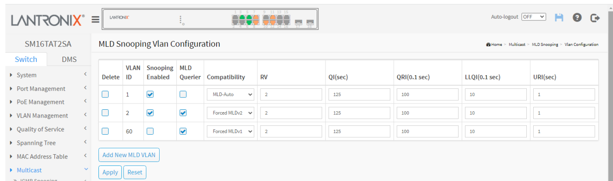
Figure 10-2.2: MLD Snooping VLAN Configuration
