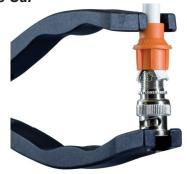
Insert the connector between the handle tips of the pliers. To terminate the connection squeeze the handles, placing your hand near the connector to obtain greater leverage.
