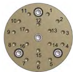
Female plug, shell size 22 (1–17 CH)
