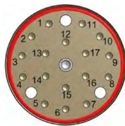
Male receptacle, shell size 22 (1–17 CH)
