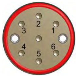
Male receptacle, shell size 16 (1–6 CH)
