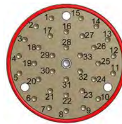
Male receptacle, shell size 28 (1–33 CH)
