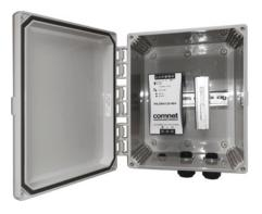
The ComNet CNEE1 Electrical Enclosure Kits provide an all-in-one solution for pole mount applications. The base CNEE1 kit includes the enclosure, mounting brackets, cable glands, and DIN rail. In the base configuration, there is  $7.297" \times 9.297" \times 6.5"$  (W  $\times$  H  $\times$  D) of space internally and the cable glands will support an AC Mains Input and up to six Ethernet or Fiber Optic cables up to 6 mm in diameter each.
