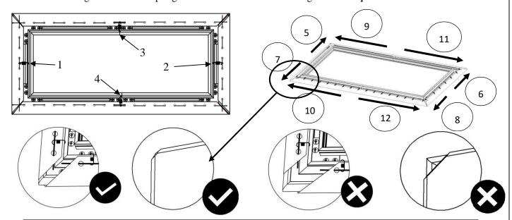
To avoid ripples forming in the material it is imperative that all the corners are properly wrapped around the edges as illustrated in the check mark diagrams.
