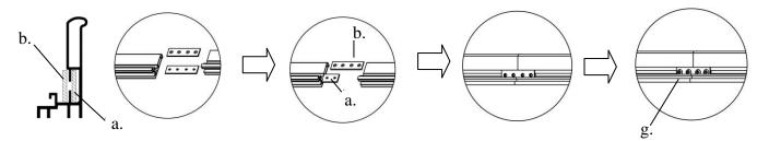
**Step 4:** Connect the *elbow joints* (*c/d*) to the top and bottom sections of the vertical frame. Once inserted, connect the vertical sections to the horizontal frame sections. Make sure all holes are in alignment and the frame pieces are flush (no gaps). They should form perfect right angles.
