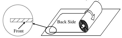
**Step 7:** Insert the rods(r) through the holes according to their corresponding lengths on each edge of the screen material as shown below. The short rods (top/bottom) will overlap to secure a firm grasp in the middle areas.
