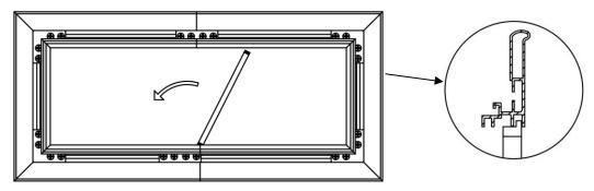
**Step 10:** Hook one end of the spring and secure inside the groove of the frame, use the *spring hook* (h) to attach the spring to the exposed part of the rod (r) in the following order.
