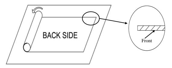
**Step7**: Carefully place the screen on top of the assembled frame as shown below.
