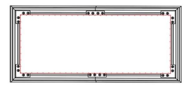
**Step 8:** Insert the *rods* (*r*) through the sleeves according to their corresponding lengths on each edge of the screen as shown below. The short rods (top/bottom) will overlap to secure a firm grasp in the middle areas.
