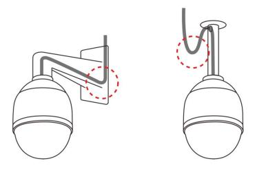
To ensure a watertight seal, the cable entry hole of the outdoor mounting kit needs to be sealed with thread seal tape to avoid water from entering the camera.
