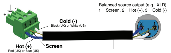
Fig.8 Balanced wiring (US).
