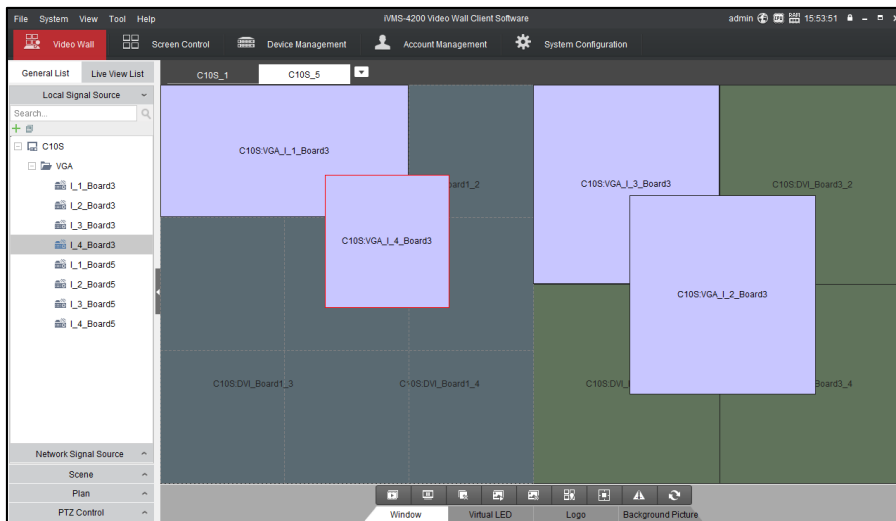
Figure 4-39 Display Signal Sources on Video Wall
