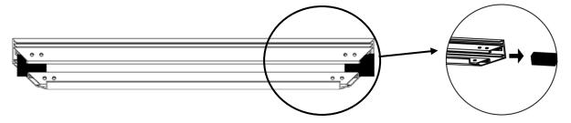
**Step 4.** Insert the center joint connectors into one-half of the horizontal frame and secure with the M4x6 screws (2 for both top and bottom). Once secure, connect the other half of the horizontal frame and fasten with the M4x6 screws (2 for both top and bottom).
