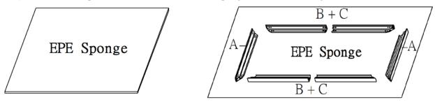
**Step 3.** Remove the foam in all frame ends before assembling the frame
