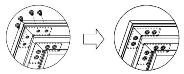
**Step 8**. Before getting started, position all the springs on the marked areas on the frames so they are near the grommet holes on the screen material. This step is very important as it will be a bit challenging to move the spring hooks once the material is completely unrolled on the frame.
