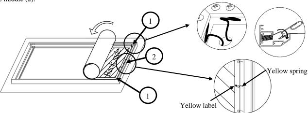
Carefully unroll the material to the middle area then hook the yellow spring on both the top and bottom (3). Continue unrolling the entire material to the other end, hook the springs in the corners (4) and hook the yellow spring in the middle (5).
