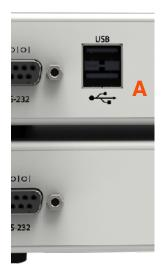
The ZyPer4K Decoder device can be ordered with optional USB connectivity.
