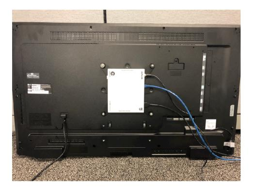
Example mounting ZyPerK to side of 200x200 VESA bracket using 2 mounting holes/screws. This *may* enable use of wall mounting bracket hardware.
