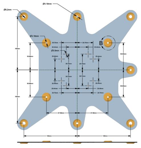
Example mounting ZyPer4K to center of 200x200 VESA bracket using all 4 mounting holes/screws. This would prevent the use of wall mounting bracket hardware.
