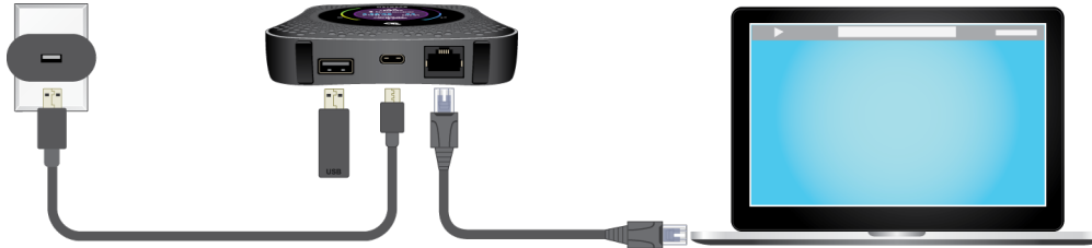
Figure 5. Ethernet offloading with AC charging and a USB storage device
