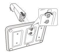
**2.** Before assembling the stand, align the groove of the connection part with the groove on the monitor to assemble them after removing the screws from the back of the monitor.
