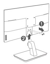
**3.** Firmly fix it in place with the screw removed from the back of the monitor.
