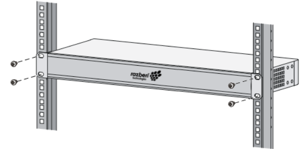
Mounting the 8 Port ServerSwitchIQ to rack posts.
