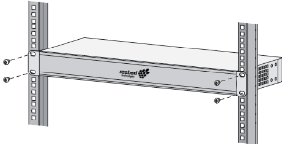
Mounting the 16/24 Port 1U ServerSwitchIQ to rack posts.
