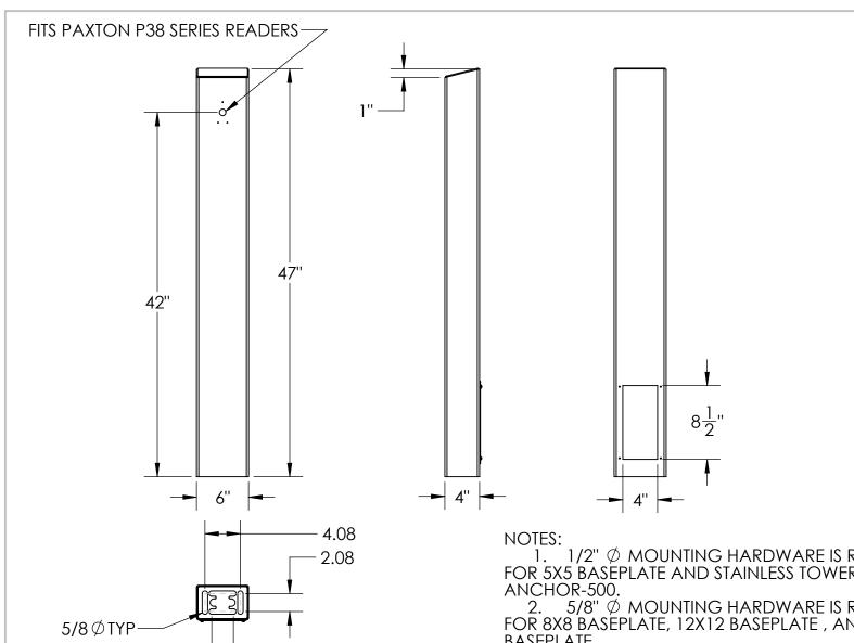
1. 1/2" Ø MOUNTING HARDWARE IS RECOMMENDED FOR 5X5 BASEPLATE AND STAINLESS TOWER MODELS. L-BOLT-500, STUD-
