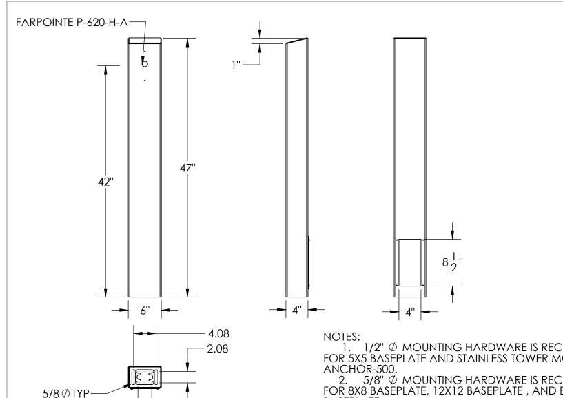
1. 1/2" Ø MOUNTING HARDWARE IS RECOMMENDED FOR 5X5 BASEPLATE AND STAINLESS TOWER MODELS. L-BOLT-500, STUD-
