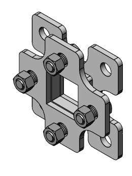
NOTES: 1. MATERIAL OF CONSTRUCTION IS MILD STEEL COATED IN 2-4 MILS OF BLACK WRINKLE POWDER COAT.
