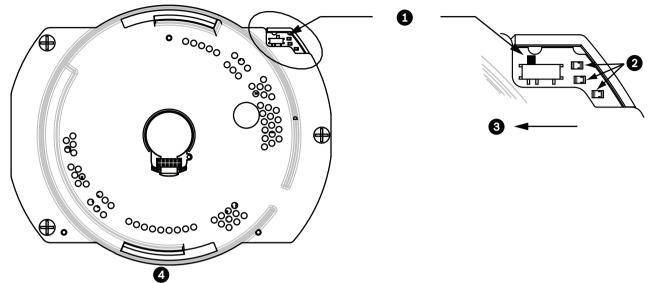
Figure 10.2: Position of CPU Switch for RS-232 Operation
