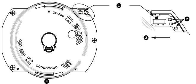
Figure 9.4: Position of CPU Switch for RS232 Operation (camera module not shown for clarity)
