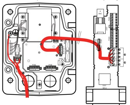
Figure 7.2: VG4-A-PSU1 or VG4-A-PSU2 Power Supply Box Connected to Pipe Interface Board
