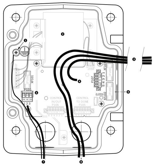
Figure 7.3: Layout of Power Supply Box. (Wire connections applicable for AUTODOME cameras.)
