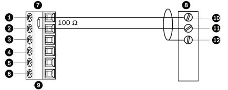
Figure 9.1: Connections for Biphase Operation
