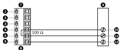
Figure 9.5: Connections for RS485 Operations
