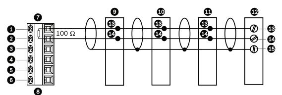
Figure 9.2: Connections for a Daisy Chain Configuration
