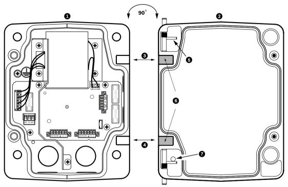
Figure 6.1: Align Cover Door Hinge to Power Box
