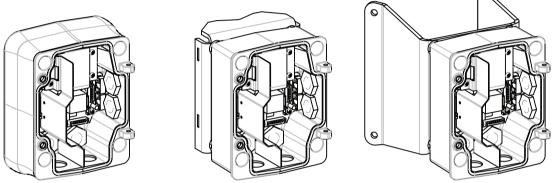
Figure 5.1: Power Supply Wall, Mast (Pole), and Corner Mounts
