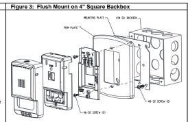
⚠ CAUTION: Do not over tighten mounting screws. Excessive torque can distort the base and may affect operation. When using power tools to screw down the mounting plate to the electrical backbox, ensure the torque is set to the lowest setting available.
