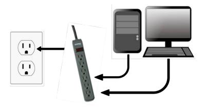
Insert the MMS362 into a utility outlet with the receptacles facing up. Next, connect your devices to the MMS362. Press the red On/Off rocker switch and verify the Red LED is activated. If so, the MMS362 is on and actively protecting your equipment. If off, press the RESET on the rocker switch. If the LED illuminates the MMS362 is operational. If the switch does not illuminate, the MMS362 may have an internal fault or has absorbed a large-enough spike to be damaged and should be replaced.
