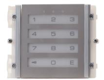
Digital electronic key module with LED keypad backlighting. Blue, white and off lighting options; stainless steel finish. When a number with between 1 and 8 digits is entered on the keypad, two relays (10A) are activated, allowing the operation of electric door locks or other devices. Dimensions 112x89.5x40 mm.
