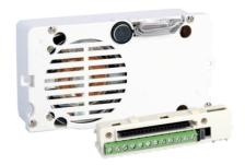
Speaker unit for 2-wire systems complete with terminal block and audio control with echocancelling, sealed-unit loudspeaker, electret microphone and front-mounted loudspeaker volume control. Complete with microprocessor and 8-position dip switch for programming calls to users. On-board electronic lock-release function (3A) plus C, NC, NO contacts for 10A relay. Timed lock-release input and door open indication. Compatible with power supply unit art. 1210. Dimensions: 102x55x38 mm.
