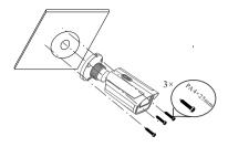
4. Bracket adjustment. Before adjustment, preview the image of the camera on a monitor and then loosen the fixed ring to adjust the view angle of the camera. Tighten the fixed ring after the adjustment.
