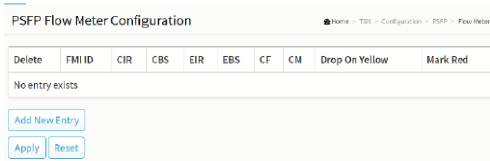
Figure 18-1.4: PSFP Flow Meter Configuration
