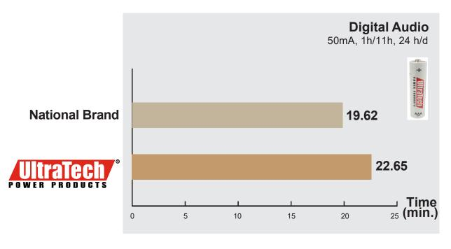
Note: Battery discharge performance evaluated by SGS in testing conditions compliant with ANSI C18.1M standard.
