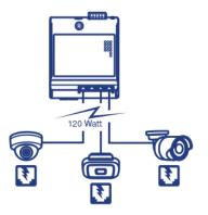
**PoE+ Power** A 120W PoE power budget supplies PoE power from the hardened industrial front access switch to up to eight Power over Ethernet devices.
