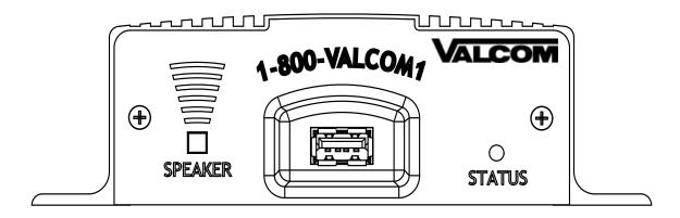
SPEAKER - The SPEAKER switch can be turned ON and OFF to monitor audio. The switch has no effect on the audio output connections on the rear of the unit. Switch should normally be kept OFF.
