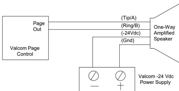
Refer to Figure 1 for audio and electrical connections. Category 3 24 AWG structured cable may be used for all connections.
