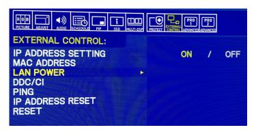
Note that LAN power is OFF out of the box so this will need to be changed for each display within the wall.
