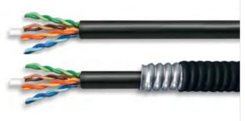
Aluminum Interlock Armor with Sunlight and Weather Resistant Polyethylene Outer Jacket (optional) Solid Annealed Copper Conductor Cross-web Separator (CAT 6 only) PFM<sup>TM</sup> Gel-filled, Water-Repellent Core Thermoplastic Insulation Sunlight and Weather Resistant
