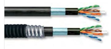
Aluminum Interlock Armor with Sunlight and Weather Resistant Polyethylene Outer Jacket (optional) Solid Annealed Copper Conductor Polyethylene Inner Jacket Rip Cord Cross-web Separator (CAT 6/6A only) PFM™ Gel-filled, Water-Repellent Core Thermoplastic Insulation Aluminum Tape Shield Sunlight and Weather Resistant
