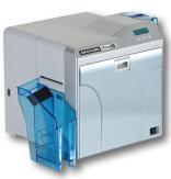
using a reverse-transfer printer, such as the Ultra Magicard Prima 4, which reverse-prints the image on a clear plastic overlay, which is then laminated onto the card. Advantages are that the printing is protected from fading or scratching by the clear plastic layer, and any card surface problems do not affect printing of the image.
