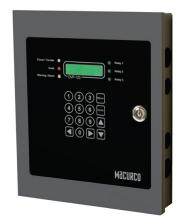
The DVP-120M is a Modbus-Enabled Detection and Ventilation Panel with up to 87 Modbus addressable sensors on three channels of 29 sensors per channel, plus the original 12 analog 4-20 mA sensor channels. The DVP-120M increases the capacity of the DVP-120 from 12 detectors to 99. System wiring includes 4-20 mA current loop and RS-485 serial interface.
