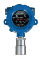
The 5100-28-IT Combustible Gas Sensor Module utilizes infrared sensor technology to monitor for combustible gases (methane and others). Output - Lower Explosive Limit (LEL) or % volume. Explosion proof, Class 1 Div. 1 Groups C, D
