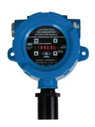
The 5100-02-IT Combustible Gas Sensor Module utilizes catalytic bead sensor technology to monitor for a wide array of combustible gases. Output range is 0-100% of Lower Explosive Limit (LEL). Explosion proof, Class 1 Div. 1 Groups B, C, D
