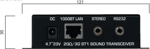
All measurements in millimeters (mm)
